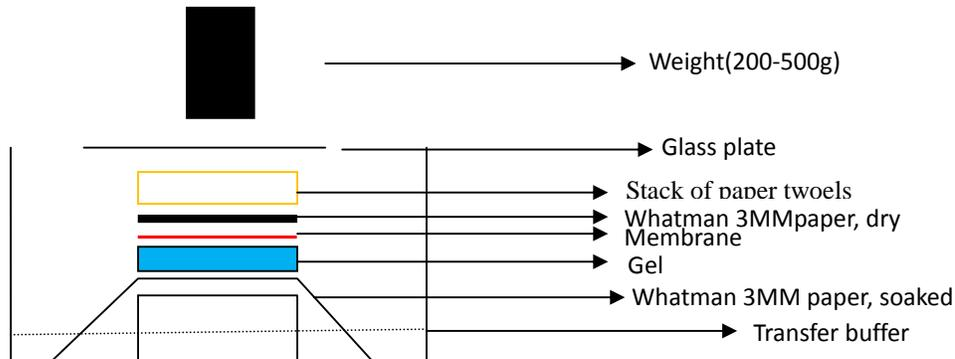
7. Allow the blot to transfer overnight in Transfer Buffer(20×SSC)
